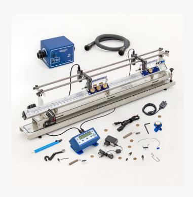
Air rail, analogue and digital multimeter, 2 photoelectric sensors and flow unit
