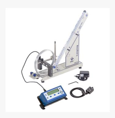
Looping with scale, magnetic hold, analog and digital multimeter with photoelectric sensor
