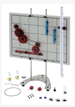
Panel with elements of machines and mechanisms - gears, pulleys and jagged bars EQ268A
