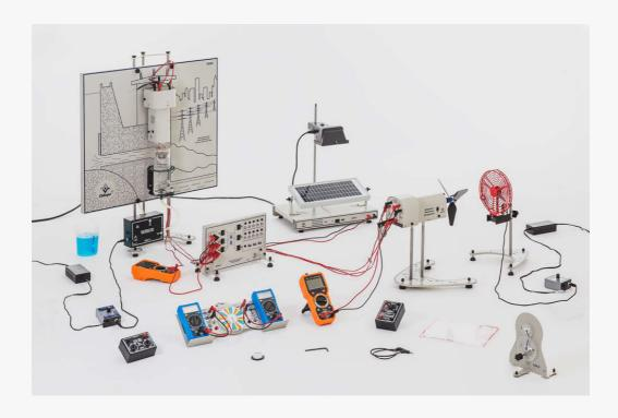
Renewable energies kit with one three-blade propeller, consumer unit and multimeter.
