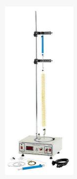
Mechanical wave kit, digital frequency meter, electromagnetic transducer and tension measurement
