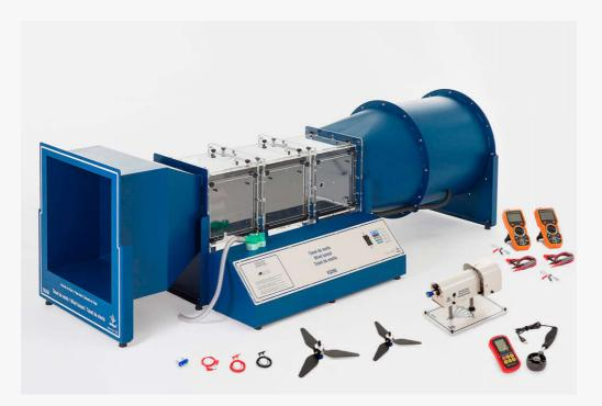
Wind tunnel with wind turbine, renewable energy, sensors and multimeters EQ266B
