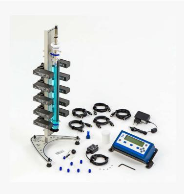
Stokes viscometer, analog and digital multimeter, 5 photoelectric sensors, 1 tube
