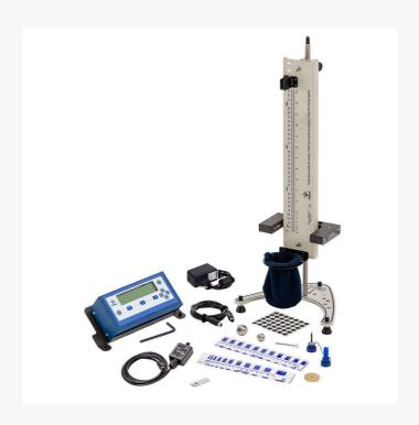
Free fall set, fences and spheres, analog and digital multimeter, photoelectric sensor
